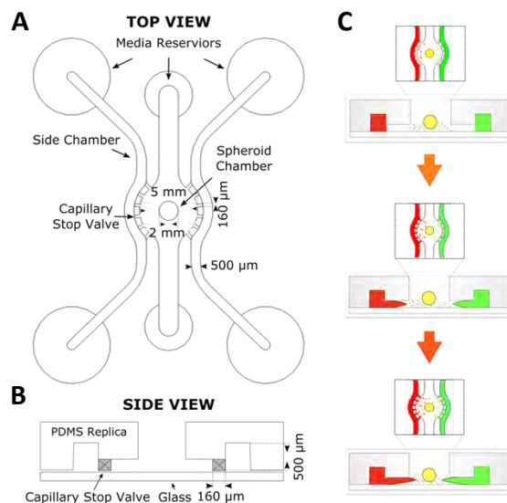
**Figure 1:** (A) Top view and (B) side view of co-culture device. (C) Co-culture workflow for mimicking the *in vivo* cancer-stromal configurations.
